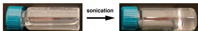
Figure 2. Gels of 1c (12 mg) form in benzene (1 mL) with sonication for 5 min at rt.
